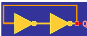
Fig.1: Simplest realization of feedback circuit
